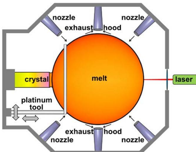
Fig. 3. Schematically represented conception of the crystal growing, with combined aerodynamic (exhaust hoods and nozzles by high-clean gas flows) & mechanical stabilization (platinum tool with the loop) of melt heated by laser through the sapphire window.
