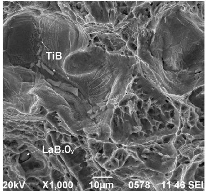
Fig. 2. Picture of surface destruction in Ti-6Al-4V/LaB<sub>6</sub> composition (secondary electron image).
