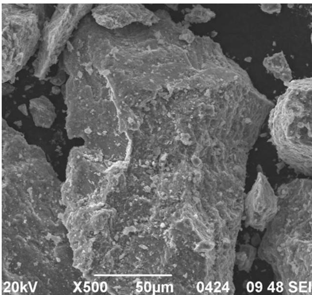
Fig. 1. The surface of powder titanium hydride (secondary electron image).
