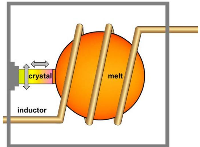
Fig. 4. Schematically represented conception of the crystal growing, with combined electromagnetic & mechanical stabilization (adjustment of the seed crystal) of induction heated melt.
